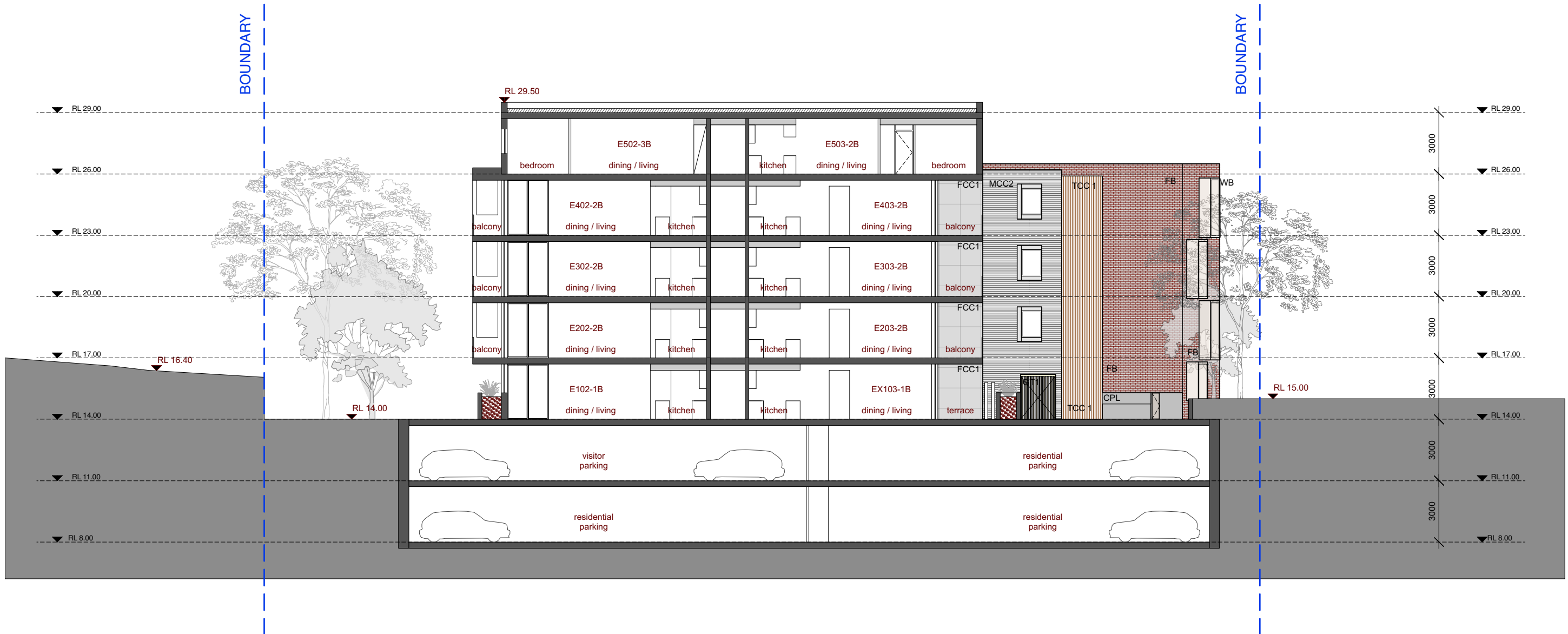
2 A-402 E-W SECTION THROUGH BUILDING E
